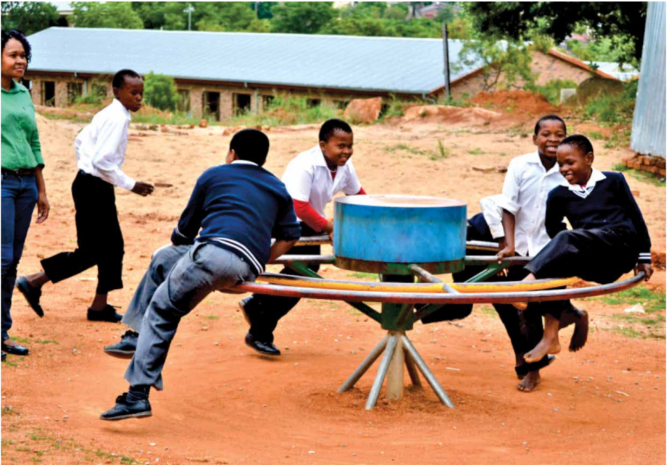
Roundabout PlayPumps provide recreational tools for children to play at, while it pumps clean water.
