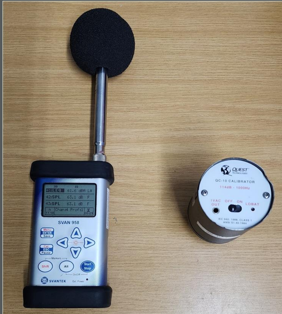
Integrated Sound Level Meter Class 1 Instrument in SANS 61672-1
