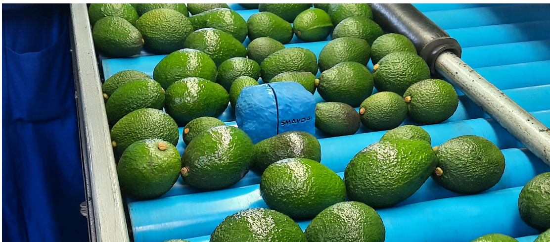
Figure 2: Avo mimicking data logger devices equipped with the latest microchip technology are proving highly effective at finding the weak links in handling procedures in the packhouse.
